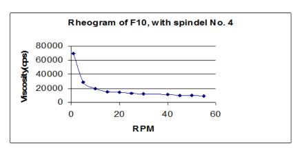
Figure 11. Rheogram of F10 with Brookfield Rheometer, Spindel No. 4 in 24°C
