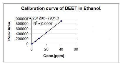
Figure 2. Calibration curve of DEET in ethanol
