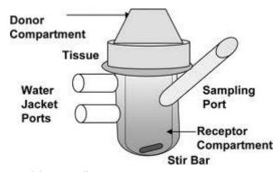
Figure 4. Schematic image of franz cell
