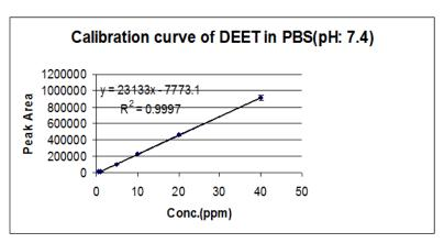
Figure 3. Calibration curve of DEET in PBS
