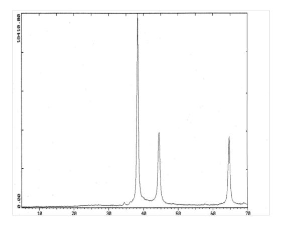
Figur 2: In XRD model, peak samples at 38, 44 and -64.5 degrees represents existence of nanosilver
